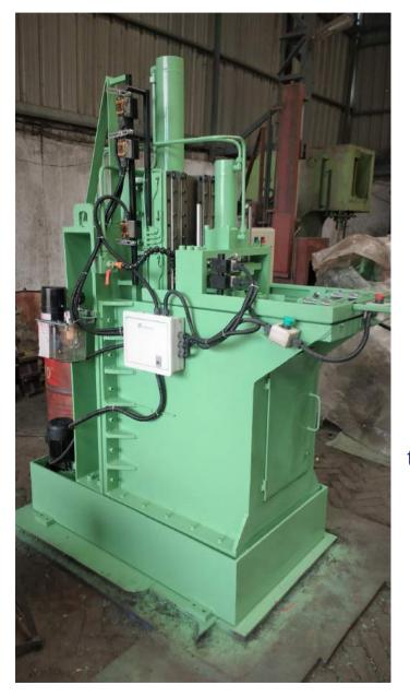
Generally used for Automotive and Heavy Engineering industries for broaching of external surfaces like matching surfaces of connecting rods,
